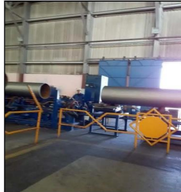
Photo.4. coating pipe gas polyethylene in Petro jet plant, port said. Source: field study, 17 april.2019
